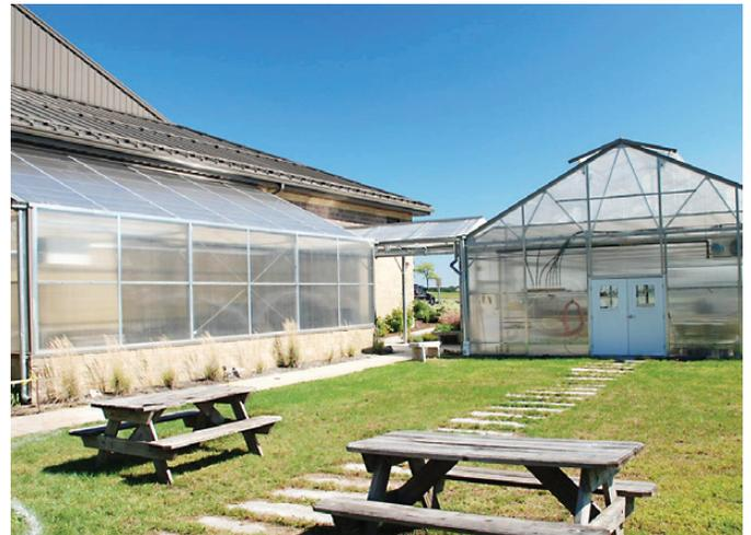
FIG. 5 Freestanding conventional greenhouse (R) and attached/lean-to (L) school greenhouses.
